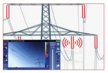
If you have installations that are more than 40 feet high, you could use the Ultrasound Imager to locate the leaks within a few inches without climbing ladders or using lifts.
