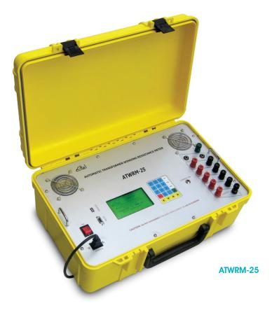
The Eltel ATWRM-25 is a high current, digital direct reading Automatic Transformer Winding Resistance Meter. It is designed to measure the DC resistance of circuits associated with large Inductances. It is specifically designed to measure the resistances of highly inductive transformer windings very quickly and accurately. The operation of the instrument is micro-processor controlled and is fully automatic.
